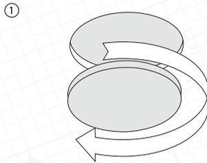
Cut out  $\varnothing$  190 mm hole for MCR 6T.
