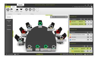
The Operator Application is used to control and operate the conference system during the meeting. The user can see and manipulate microphone activity, have a clear view on the meeting synoptic, and define the interaction of the delegates. Functionalities include:
