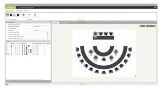
The Room Configurator is used to create and edit the room synoptic. A synoptic is a visual representation of the conference room setup. It can contain microphones, a background image, and more.
